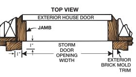
NOTE: 1" wide by 1"deep mounting surface is recommended for proper installation.
